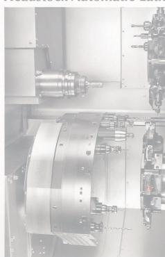
Up to three tools can be used simultaneously to produce independent contours.
