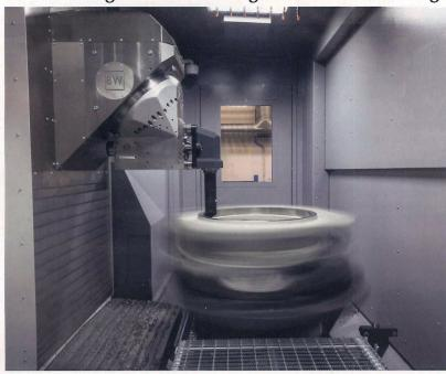
Burkhardt+Weber has expanded its model range of the multitasking MCT series with the MCT 1250. A variety of adaptable chip cutting tasks with rotating tools, like milling, drilling, boring, grinding, CNC facing, 3-D milling and more are combined with rigid vertical turning for large part sizes. The high-speed torque table with up to 1,400 x 1,600 mm (55.1" x 63.0")
