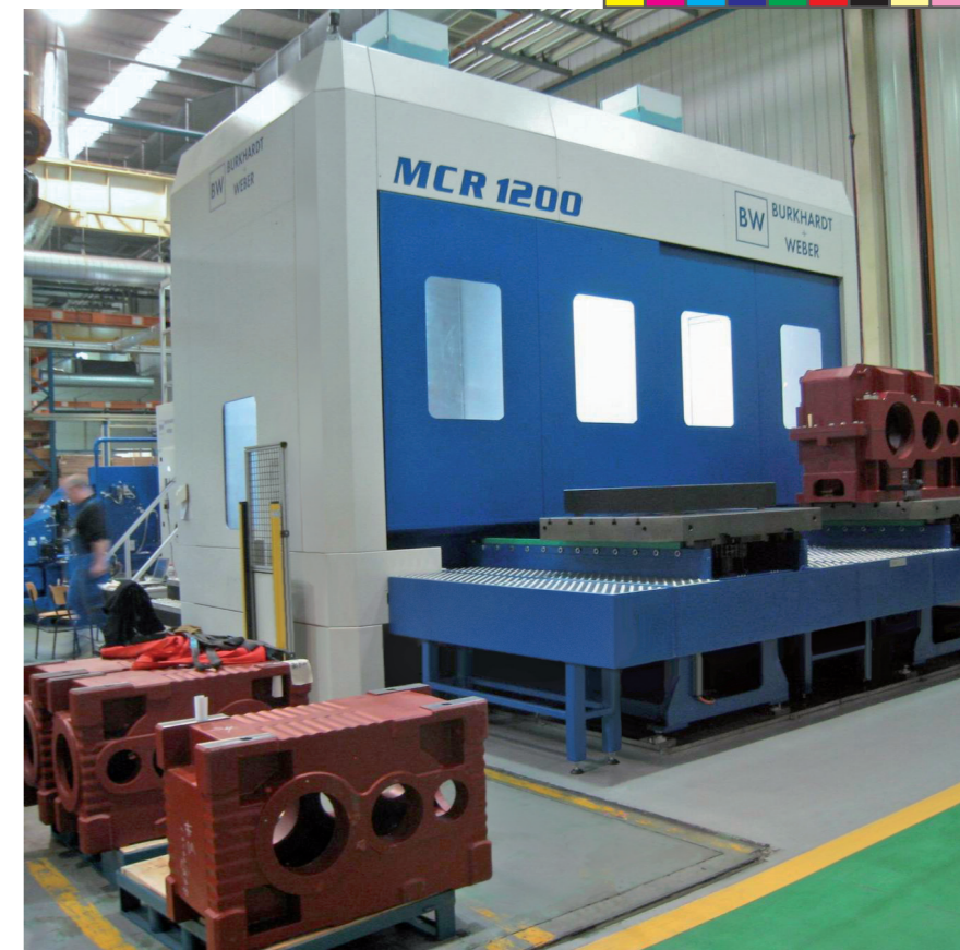
Large dimensioned and with high power at the spindle: the machining centre MCR 1200
